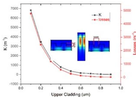
Figure 1. Simulation of losses and coupling factor vs thickness of upper cladding with a fixed etching depth of 0.3  $\mu\text{m}$
