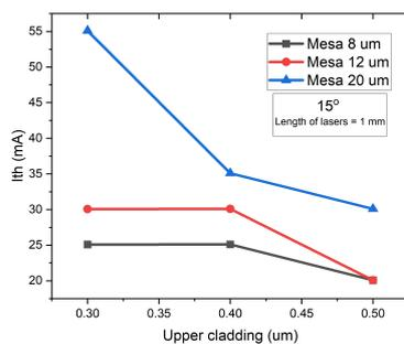
Figure 2. Threshold current  $I_{th}$  vs thickness of upper cladding for different lasers widths ( $\mu\text{m}$ )
