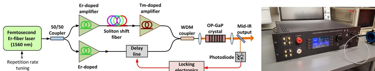
Fig. 1. Experimental setup of the DFG-based comb together with a photo of the prototype of the device.
